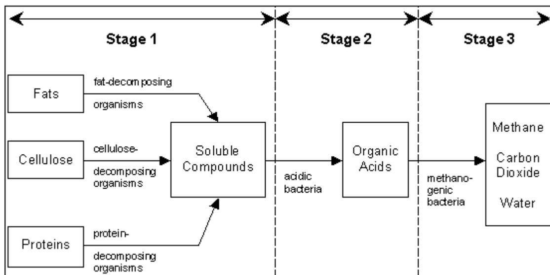
**Figure 1 Three stages in the process of anaerobic treatment**
