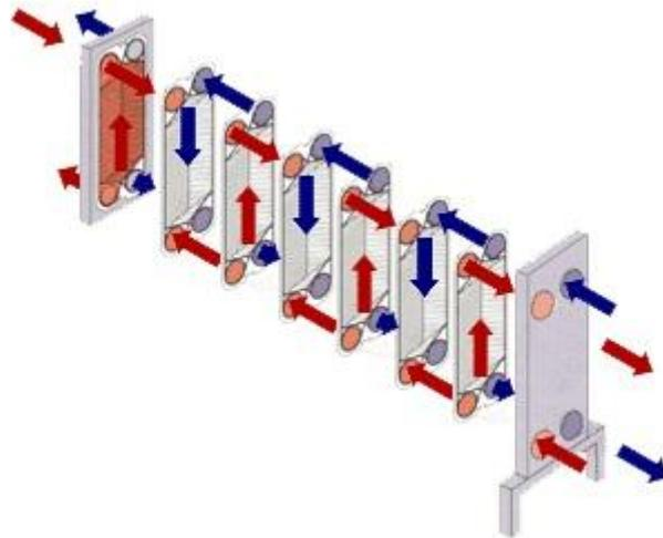
**Figure 2 Schematic Diagram of a plate heat exchanger**
